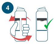
Hold filter as shown above. Firmly insert into filter head. Turn filter 1/4 to the right until it locks into place and the front label is clearly visible.
